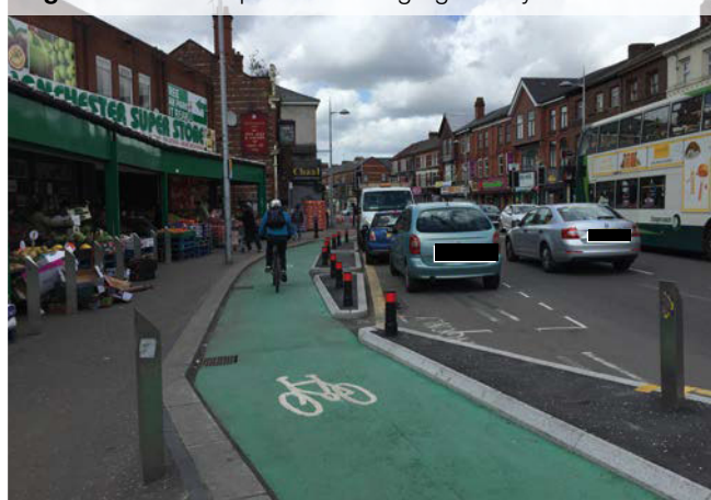
Figure 1.10: Example of kerb-segregated cycle track
