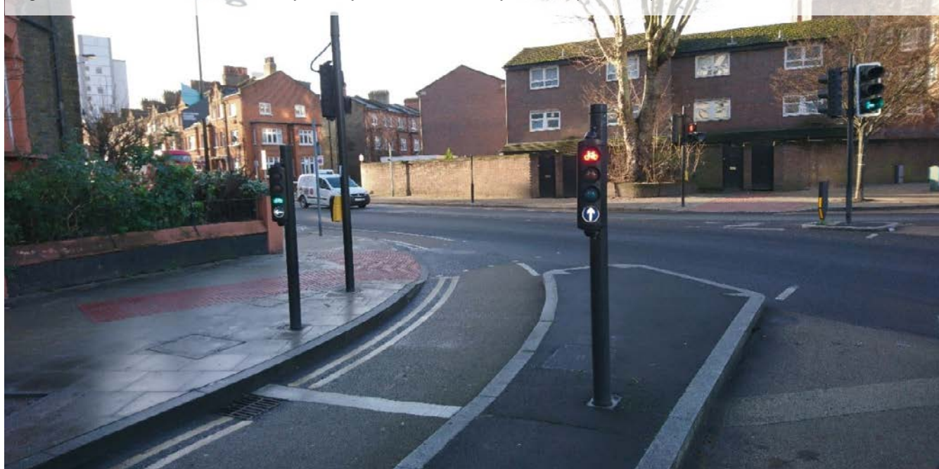
Figure 10.20: LLCS used to control cycle-only movements on a cycle track (Battersea)
